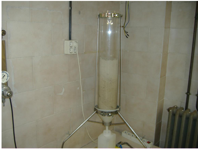
Fig. 1. Leaching column used in the laboratory experiments.
